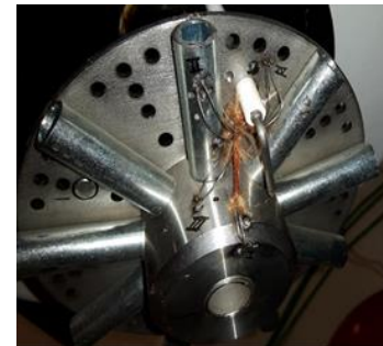
475 kw burner deck with thermocouples to monitor the temperature.
